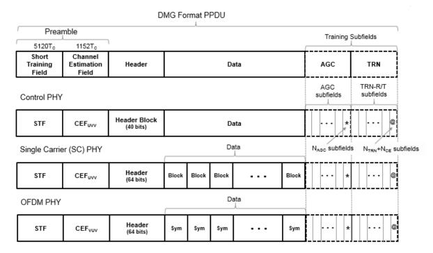
The single-carrier chip timing,  $T_{\rm C} = 1/F_{\rm C} = 0.57$  ns. For more information, see Waveform Sampling Rate on the wlanWaveformGenerator function reference page.
